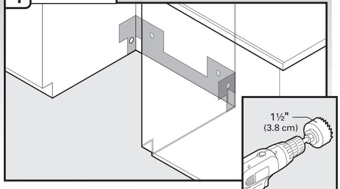
If needed, drill a  $1\frac{1}{2}$ " (3.8 cm) diameter hole in cabinet wall or side of the opening closest to the sink.
